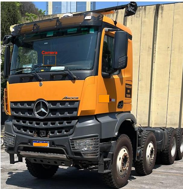
**Figure 1.** Highlighting the camera installed in the cabin of a Mercedes Arocs truck.
