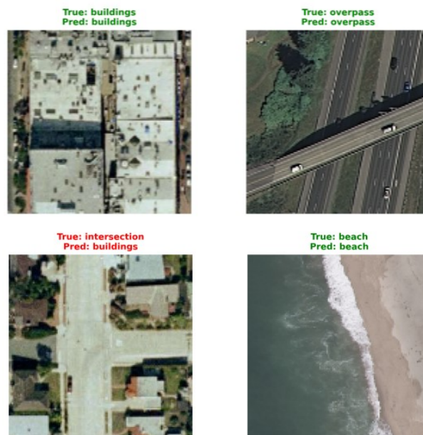
Figure 10. Sample predictions from the fuzzy membership classifier showing correct classifications (green) and misclassifications (red)
