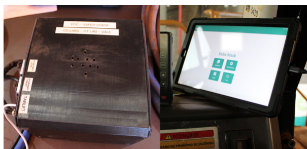
Figure 4. Encapsulation with the on-board computer and the graphical interface.
