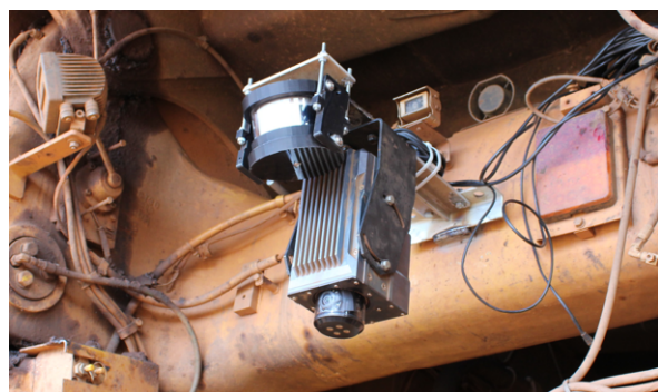
Figure 3. Camera and LiDAR installed on dump truck.
