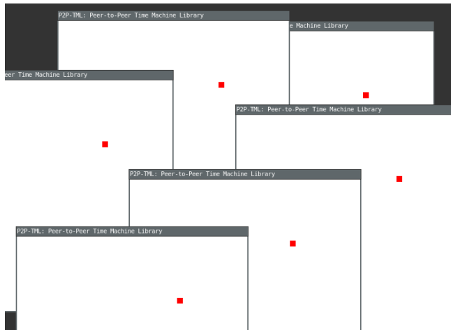
Figure 3. A moving rectangle is controlled by peers connected indirectly. Users can press \uparrow \downarrow \rightarrow \leftarrow to change the direction of the rectangle or SPACE to pause the application. The inputs are applied simultaneously in all peers, as if they were mirrors of a single application. Video: https://youtu.be/zkl0vSOGino
