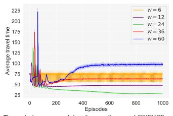
**Figure 4.** Average travel time for non-discounted SWPUCB with different values of *w*.
