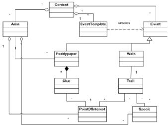
Figure 2: Domain Model of the eXciting Trails/Events system.
