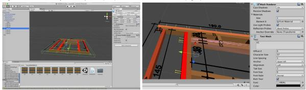
Figure 9 - Smartphone (left) and Epson Moverio™ BT200 (right) use for visualization of the wood-frame wall
