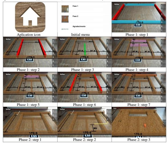
Development of an Augmented Reality environment for the assembly of precast wood-frame wall from the BIM model 69
