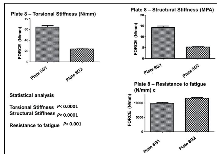
**Figure 11.** Comparison between groups G1 and G2, where the 11 mm plates differed significantly for flexural stiffness ( $P < 0.0001$ ) and structural stiffness ( $P < 0.0001$ ). However, there was no statistical difference for structural strength. These results show that the non-molded plates presented better results than the molded plates, except for the flexural resistance test, in which the two groups presented similar results.
