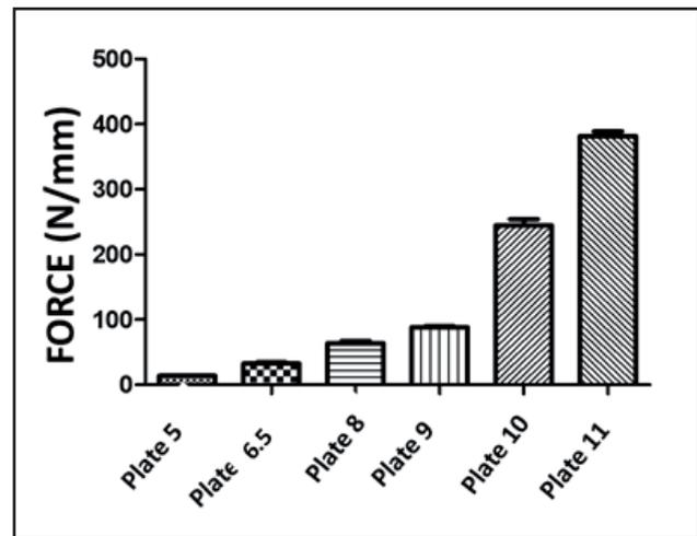
Figure 3. Comparison of all plates according to flexural stiffness. In group 1 of unmolded plates, the 5 mm plate presented the lowest resistance and the 11 mm plate presented the highest resistance. In group 2, when comparing different resistance plate sizes, 5 mm and 11 mm plates also had the lowest and highest resistance, respectively.
