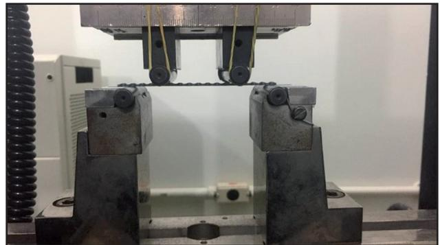
**Figure 2.** The flexion testing machine.
