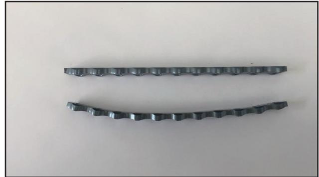
**Figure 1.** Titanium orthopedic plates (8.0 mm), the first (from top to bottom) in group 1 without molding, and the second in group 2 with molding to the dog femur bone.
