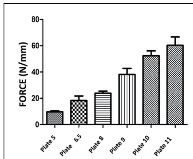
Figure 4. Comparison of all plates in each group. The 5 mm and 11 mm plates had the lowest and highest resistance, respectively.
