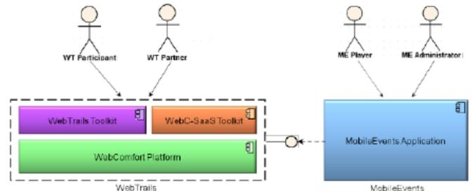
Figure 1: Overview of the system's components
