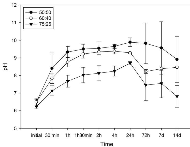
Figure 2: Mean pH values for different cements after immersion in distilled water over different times.
