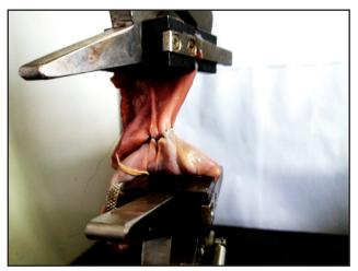
Figure 3. Tensile test on the EMIC 23-5D tensiometer.
